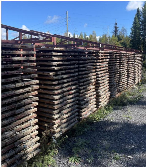
Figure 10.5 – Example of Core Rack Arrangement
