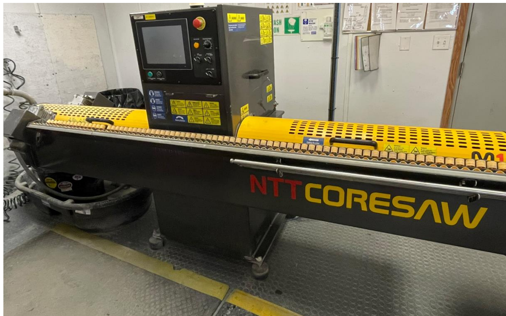
Figure 10.10 – Automated Diamond Core Saw Setup at Musselwhite
