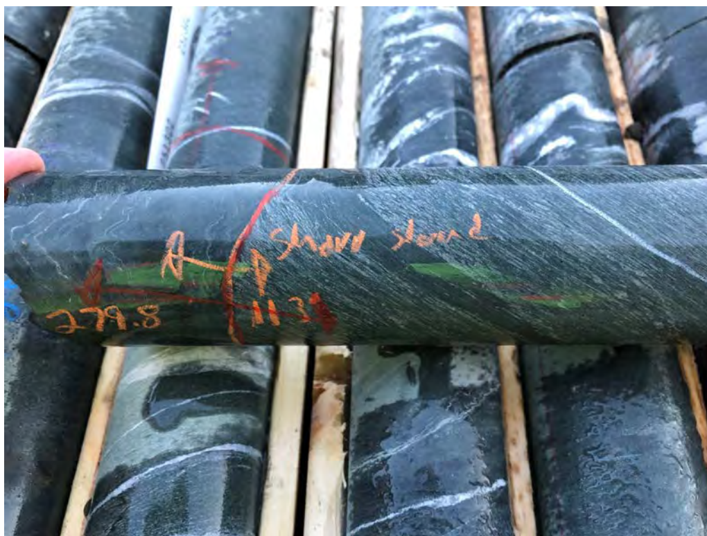
Figure 7.6: Contact of Sheared Gabbro (right) with BIF (left) DDH 19-52
