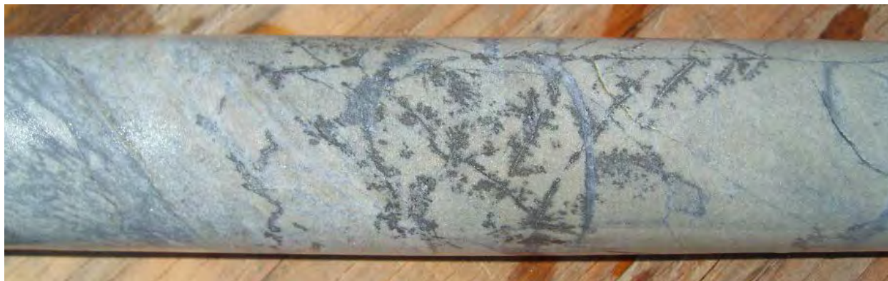
Figure 7.18: Example of Fracture-controlled Pyrite Mineralization in Sericite-silica Arkosic Wacke, 0.54 ppm Au
