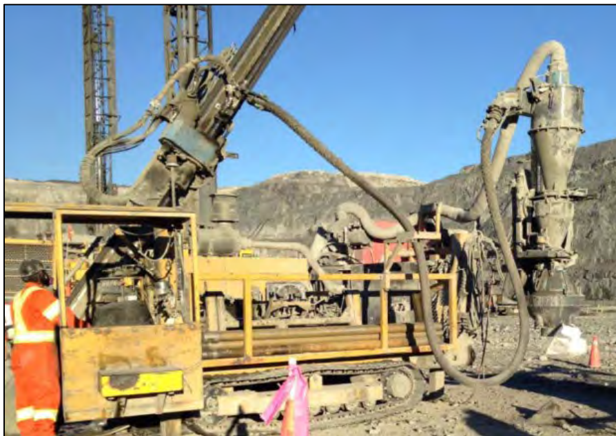
Figure 10.5: Hardab 7000 Maxidrill RC Drill Rig
