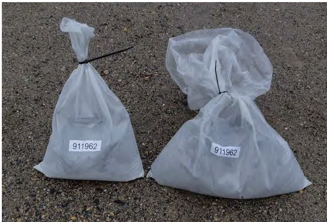
Figure 11.1: Principal Sample (small) and Metallurgical Sample (large) from a 2 m Interval - RCGC Sample
