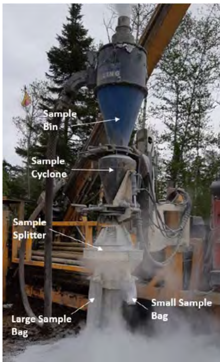
Figure 11.2: Hardab 7000 Maxidrill RC Drill Rig and Splitter in Operation
