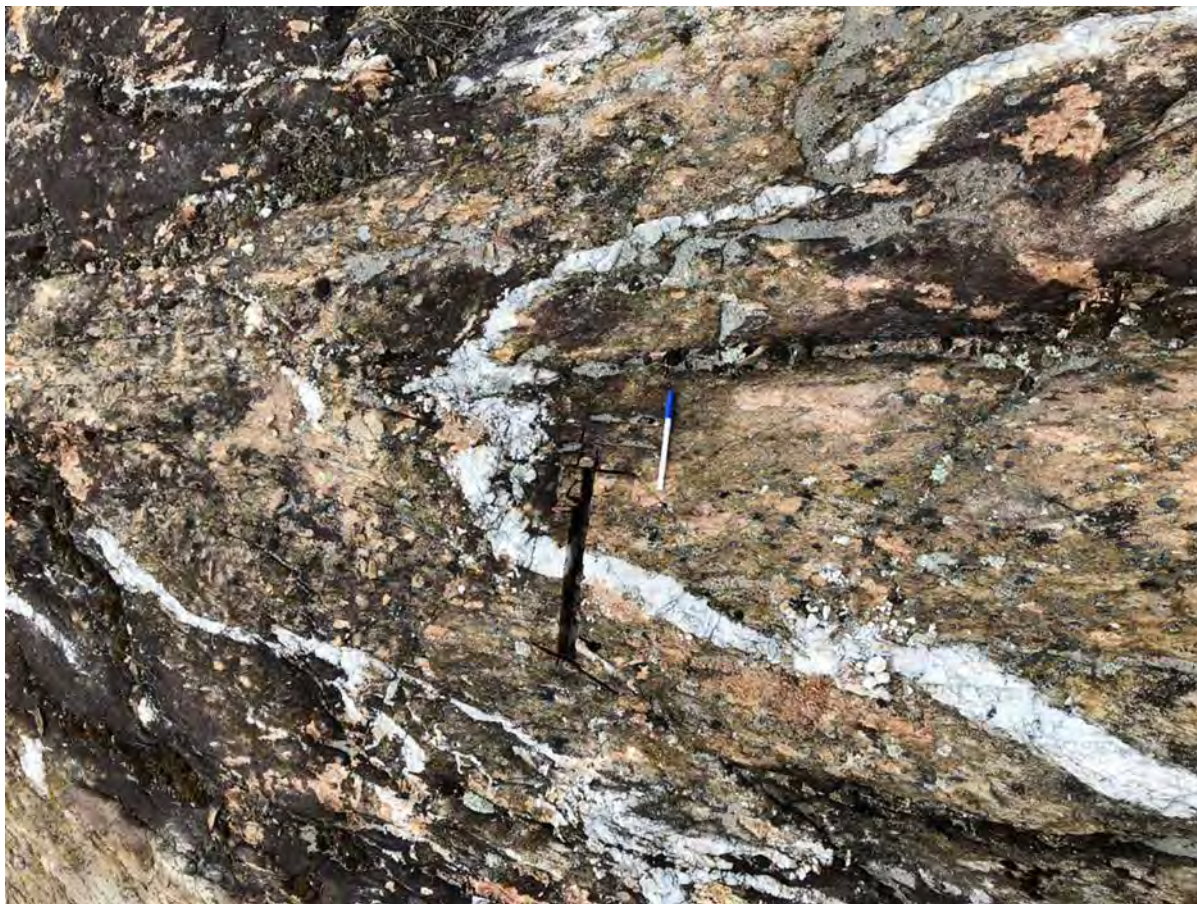
Figure 7.13: Folded Quartz-carbonate Veins within Altered Quartz-porphry, Porphyry Hill
