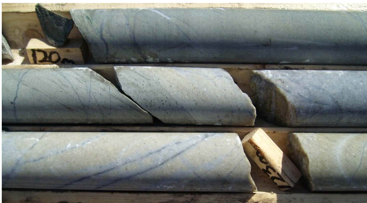
Figure 7.19: Example of Sericite-altered Quartz-feldspar Porphyry; 7.75 ppm Au. Dyke Intrudes Arkose (top core)
